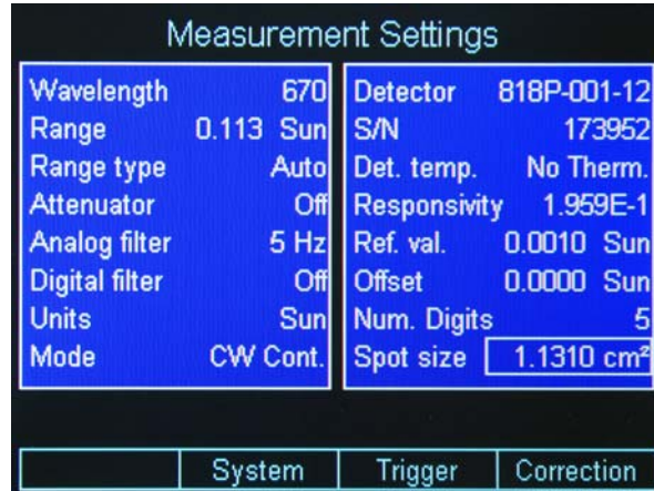
Figure 19 Measurement Settings screen
