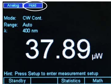
Figure 26 Measurement is on hold
