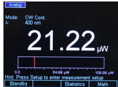
Figure 48 Analog Needle display
