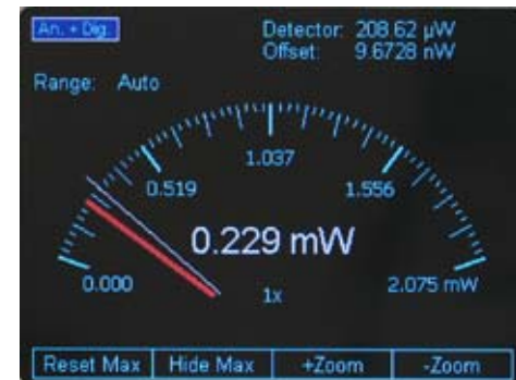
Figure 52 Analog Gauge Display with Maximum Value marker
