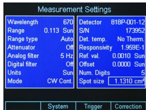
Figure 32 Measurement Settings screen
