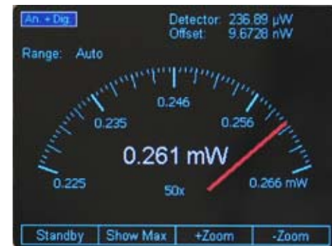
Figure 53 Analog Gauge Display at 50x Zoom
