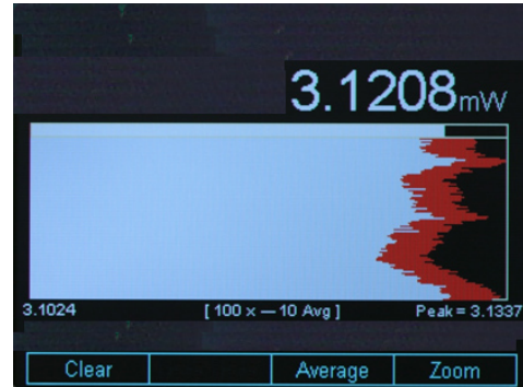
Figure 49 Vertical chart with 10 measurements per line
