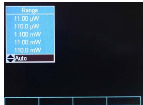
Figure 24 This screen is displayed after pressing the Config soft key
