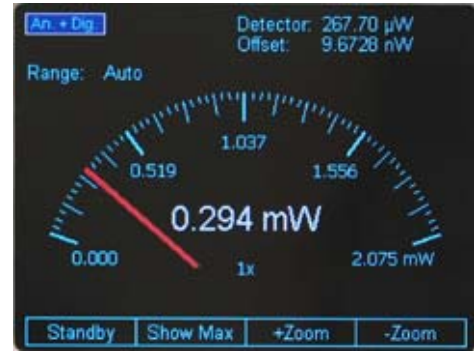
Figure 51 Analog Gauge Display
