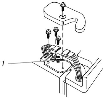
4. Disassemble right top hinge.
