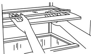
3. Replace back of meat drawer cover frame into supports on side walls of the refrigerator and lower the front of the cover frame into place.
