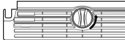
2. Remove the cartridge cap by sliding it off the end of the old cartridge. The cap will slide to the left or right. **DO NOT DISCARD THE CAP.**
