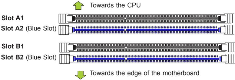
The X10SLH-F supports up to 32GB of Unbuffered (UDIMM) DDR3 ECC 1600/1333 MHz (1.35V/1.5V) memory in 4 slots. Populating these DIMM modules with a pair of memory modules of the same type and same size will result in interleaved memory, which will improve memory performance. Please refer to the table below:
