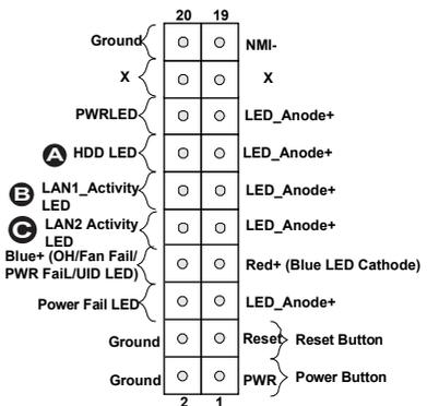
**Overheat (OH)/Fan Fail/PWR Fail/UID LED**
