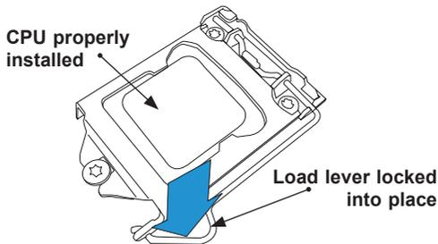
**Warning:** You can only install the CPU inside the socket only in one direction. Make sure that it is properly inserted into the CPU socket before closing the load plate. If it doesn't close properly, do not force it as it may damage your CPU. Instead, open the load plate again and double-check that the CPU is aligned properly.
