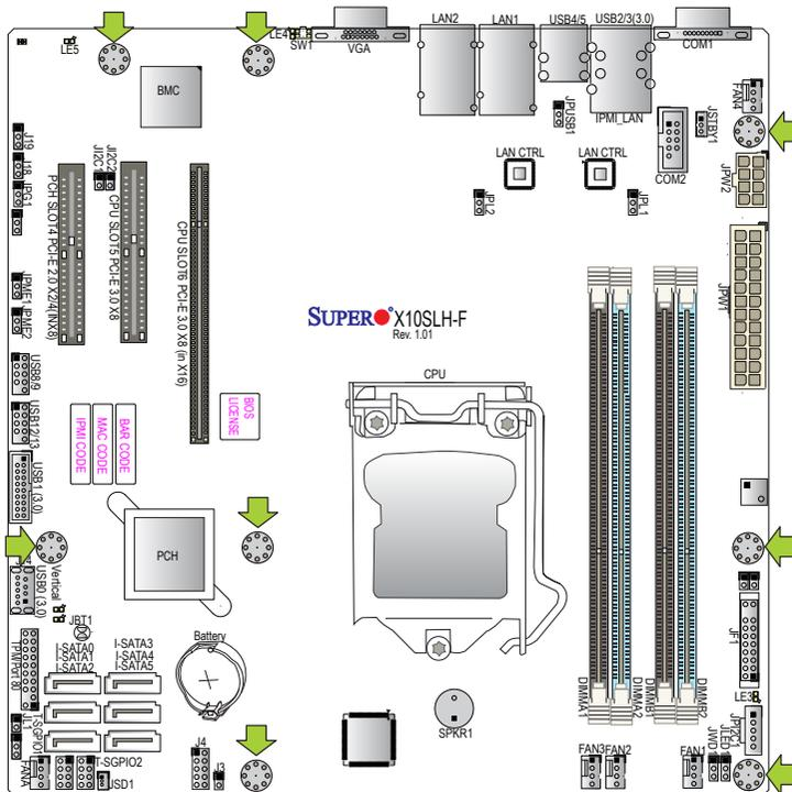
**Caution:** 1) To avoid damaging the motherboard and its components, please do not use a force greater than 8 lb/inch on each mounting screw during motherboard installation. 2) Some components are very close to the mounting holes. Please take precautionary measures to avoid damaging these components when installing the motherboard to the chassis.
