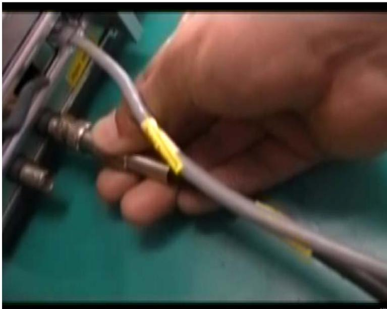
Fig 7 Connect “Visual Video 1” connector onto corresponding interface “Visual Video” on PC
