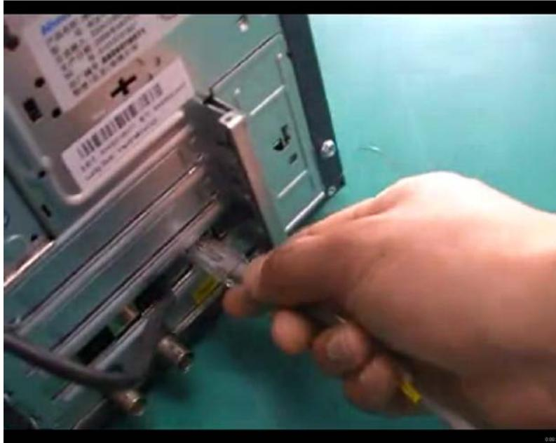
Fig 3 Connect RJ45 connector to the network interface on 1801A card
