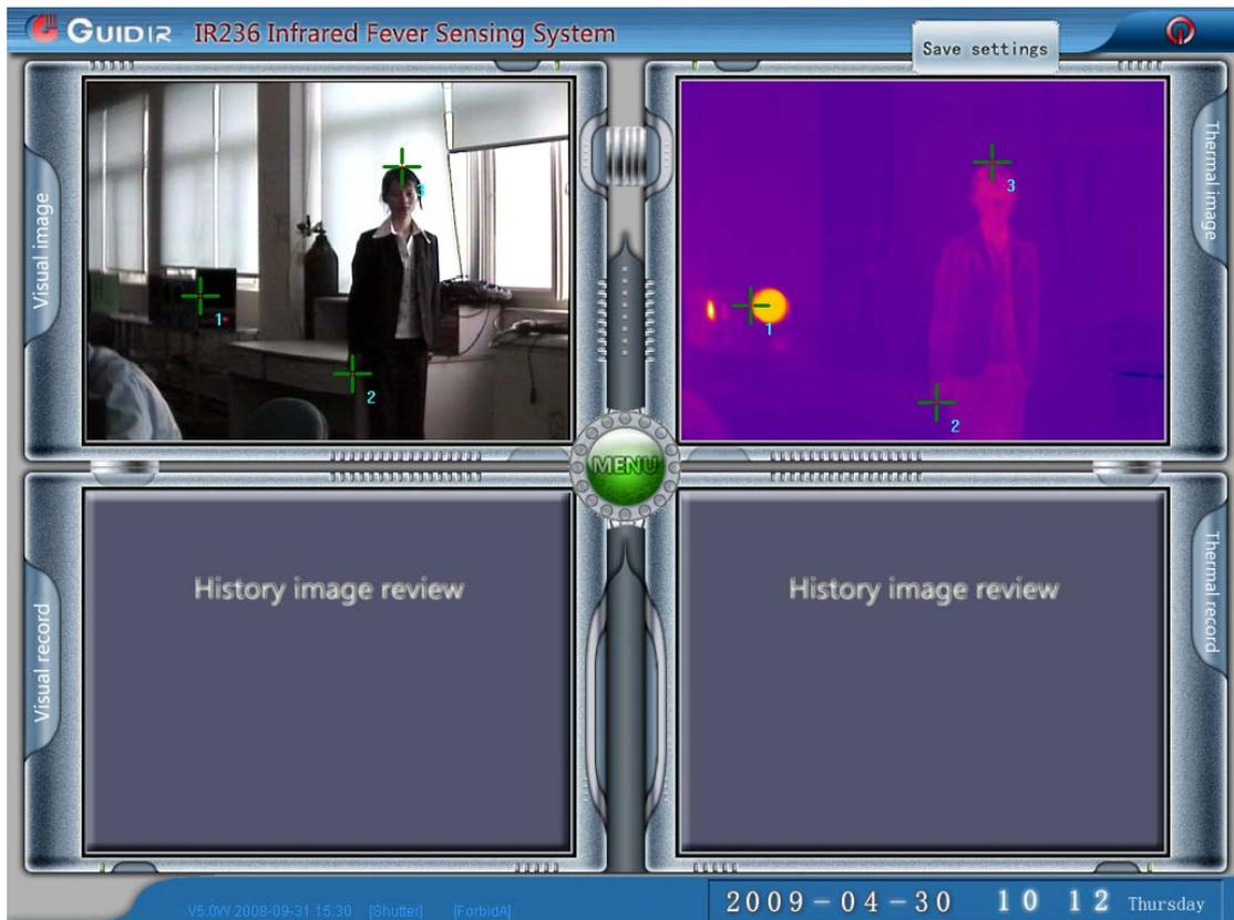
Figure 2-12 Position of the three aligned spots
