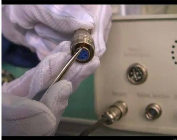
Fig 2. Please notice there is a small gap on the “Digital Interface” connector, which needs to be aimed at the gap in “Digital Interface” on the camera body.
