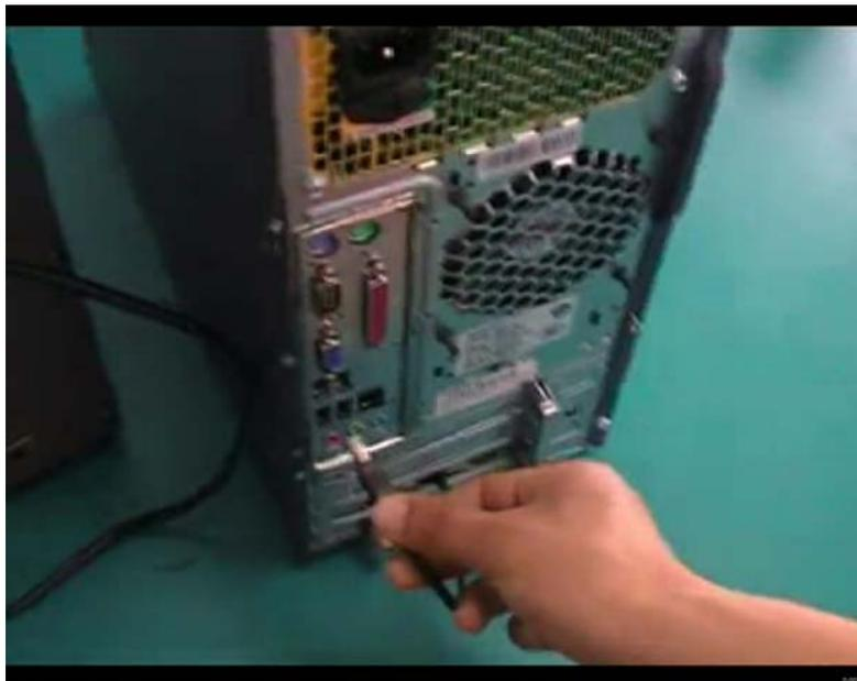
Fig 2 Connect USB cable of 1801A card to USB interface of PC.
