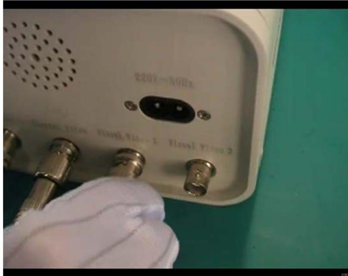
Fig 2. Aim the connector at the interface, press and rotate the connector until it reaches the correct position.
