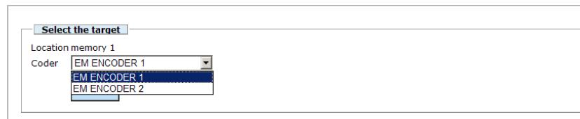
1. Select the Basic encoder that is to receive the configuration.
