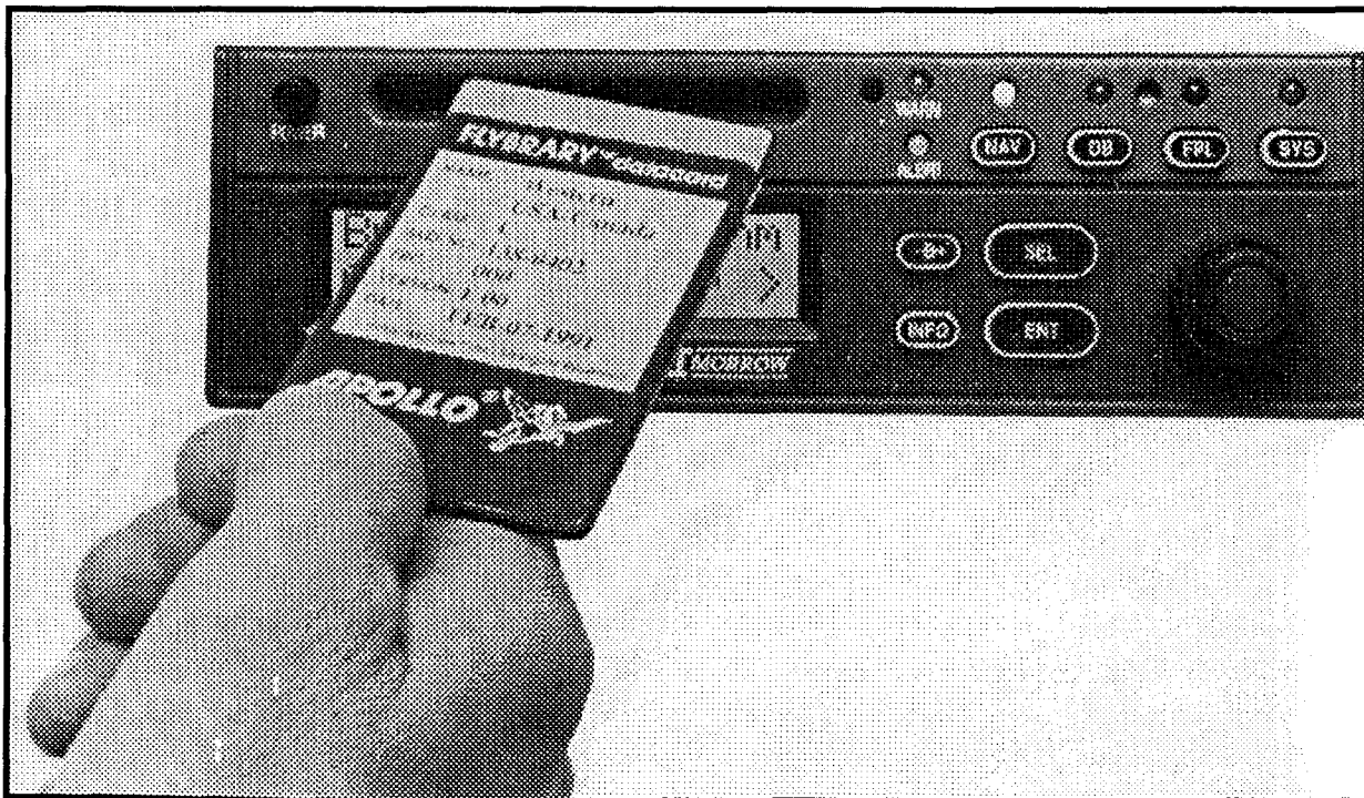
Datacard being inserted into aviation laser receiver. Datacards can be periodically replaced to ensure the database is current.
