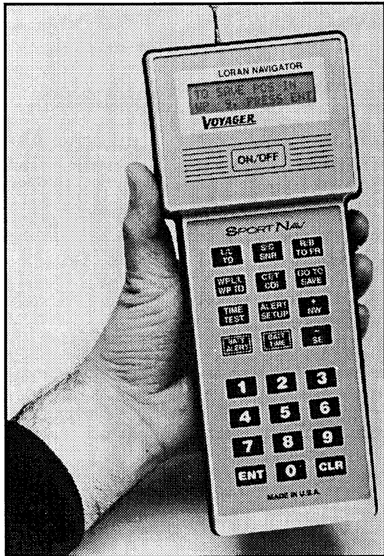
Example of a “hand held” loran powered by 6 AA batteries. The antenna is telescoping and no external ground is required.
