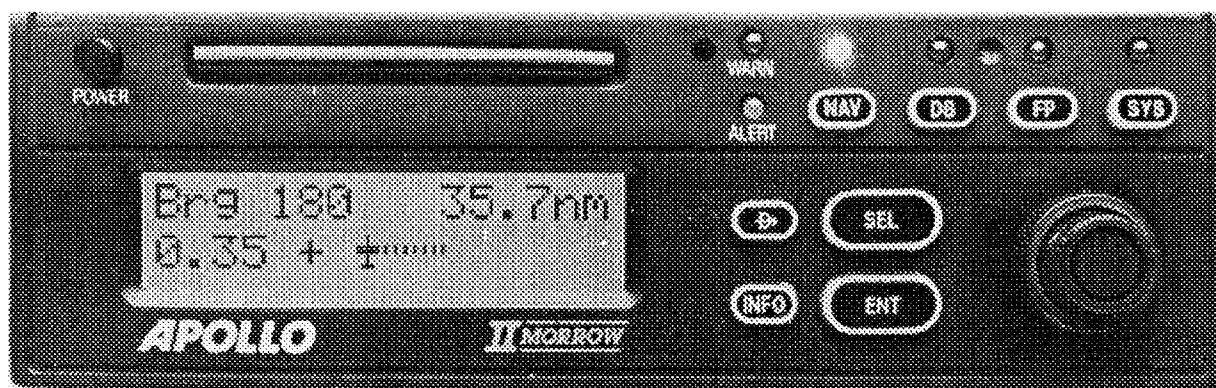
Aircraft loran displaying bearing and distance to waypoint. The second line shows the magnitude (0.35NM) and direction of the XTE.
