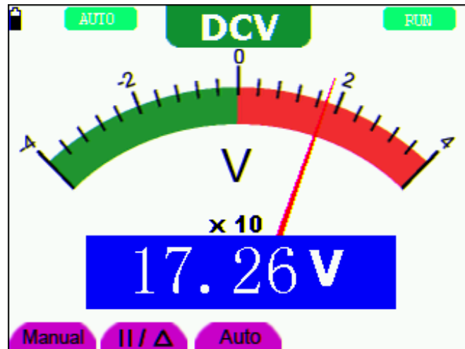
Figure 24: DC Voltage Measurement
