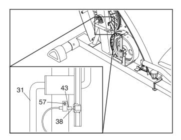
Slide the Reed Switch (43) slightly closer to or away from the Magnet (38), and then retighten the M4 x 16mm Screw (57). Turn the Crank (31) for a moment.
