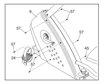
Next, remove the M4 x 16mm Screws (57) and the M4 x 25mm Screw (45). Then, carefully remove the Left Shield (9).
