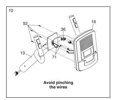
While a second person holds the Upright (13) near the Frame (1), connect the Upper Wire (36) to the Lower Wire (8).
