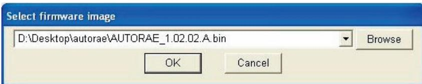
The utility will automatically select a firmware file. Ensure that this is the correct firmware file. If it is not, click on the **Browse** button and navigate to the appropriate file and click on the **Open** button:
