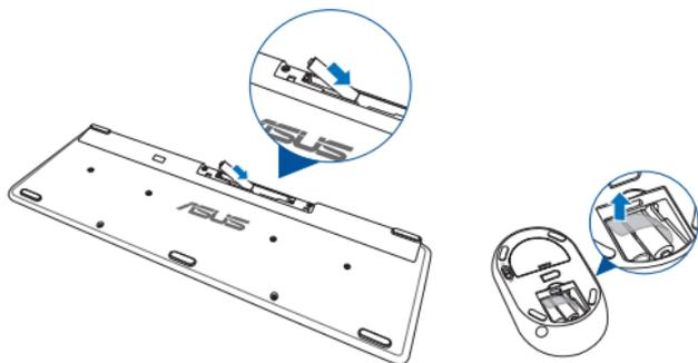
2. Connect the wireless dongle for keyboard and mouse to the USB 2.0 port to automatically pair both devices to your ASUS All-in-One PC.
