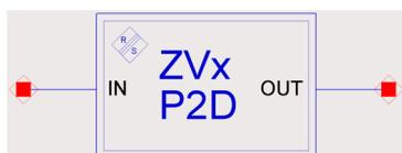
The component will control a Vector Network Analyzer and create an S parameter file for a 2-Port DUT. Additionally, the power at the ports will be swept according to the settings.
