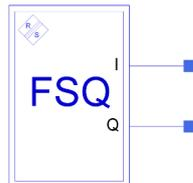
The FSx\_IQ\_Source model downloads data from any of the R&S FSIQ / FSP / FSUP / FSU / FSQ / FSG / FMU36 / FSW / FSV/FSL Spectrum and Signal Analyzers into ADS. It outputs IQ data as recorded from the detector.
