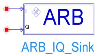
The ARB\_IQ\_Sink model downloads time domain IQ data from ADS to the R&S Vector Signal Generator or Arbitrary Waveform Generator or R&S I/Q Modulation Generator.
