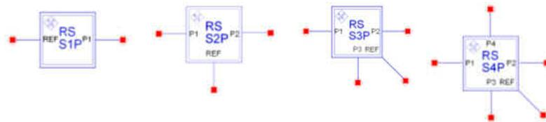
The component will control a Vector Network Analyzer and create a S parameter file for a 1-Port / 2-Port / 3-Port / 4-Port DUT.
