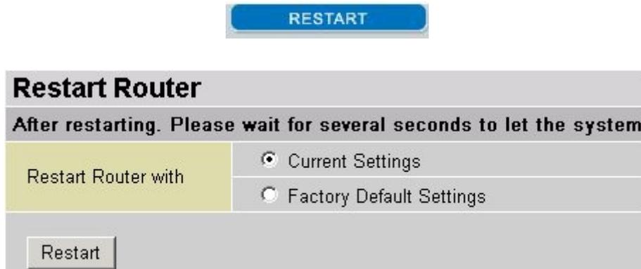
The screenshot shows a web interface for restarting a router. At the top is a blue button labeled "RESTART". Below it is a grey box titled "Restart Router" with the instruction "After restarting. Please wait for several seconds to let the system". Underneath, there is a section "Restart Router with" with two radio button options: "Current Settings" (which is selected) and "Factory Default Settings". At the bottom of this section is a "Restart" button.
