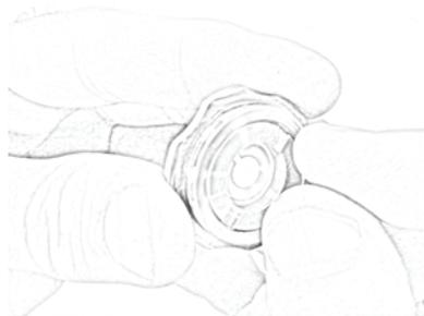
3. Remove retainer ring to access mock crystal.
