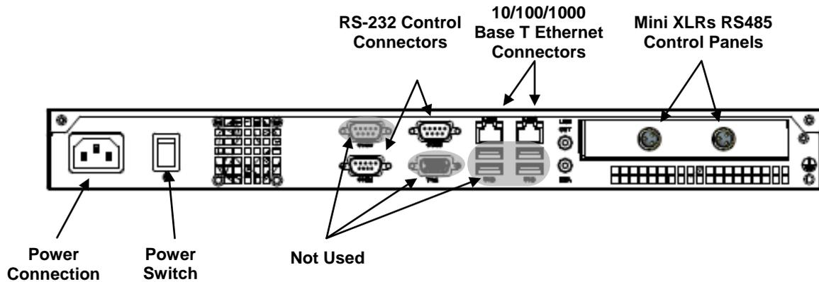
The Ethernet port labeled **LAN 1** defaults to IP address 192.168.1.225. The port labeled **LAN 2** is set for DHCP operation and must get its IP address from a DHCP server.
