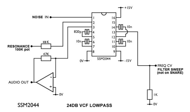
The iconic **Curtis chip SSM2044** (but also low cost) low pass filter was used to filter the noise in the SDS-V, the resonance can be tweaked but never in a big amount and you will not reach selfoscillation on the SDS-V. This is the type of filter that will not maintain the gain around the cutoff resonance, so you will lose the bottom end. The frequency CV of the filter will be affected by the
