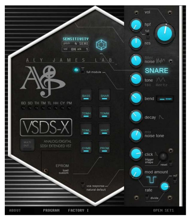
The SNARE featured 2 additional parameters, the **FULL NOISE** (which lets all the noise generator frequencies pass through) and the **VCF modulation switch** (it will send the full modulation amount to the VCF cutoff, regardless of the modulation amount). VCF modulation is applied additionally to the VCO modulation, so you will still have control over the VCO modulation.
