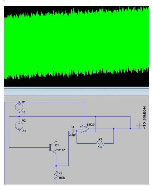
It is based on classic transistor noise amplification (transistor + OPAMP) with a special thing, the twisted wires...
