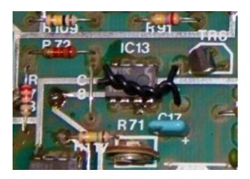
It is called a gimmick capacitor, used to get a very small pico-farad capacitance and it is here in place of a proper compensation capacitor on the op amp. It seems to let one be able to 'tune' the noise easily, this is available to tweak in VSDSX as the **HPF** knob. It lets you filter out some of the noise generator frequencies and is nice to produce a fuller noise sound, the SNARE in VSDSX have an extra setting called **FULL NOISE** which will brings all of the noise generator frequencies.
