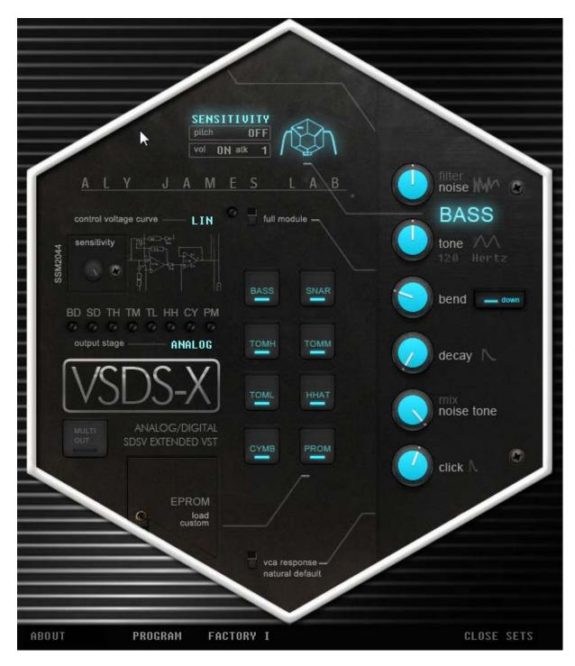
The OPEN SETS panel will let you fine tune some global parameters like control voltage curve, output stage emulation modes and SSM2044 (VCF) sensitivity. These settings affect VSDSX globally.
