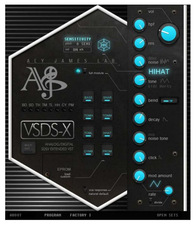
**PLEASE NOTE A PARTICULAR BEHAVIOR for the NOISE filter knob,** when set fully anti clock wise it is affected by the envelope and behaves like the BASS and TOM voice (the noise gets duller as the envelope decays). When it is set at 12 o'clock it behave like the SNARE voice (cutoff is not affected by the envelope) and when set fully clock wise, the noise starts dull and gets brighter as the envelope decays.
