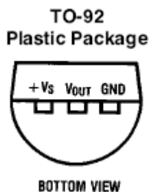
Figure 2.5 Plastic package bottom view of LM 35
