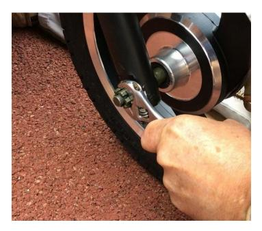
Remove the front axle, fit the front wheel onto the axle and tighten securely
