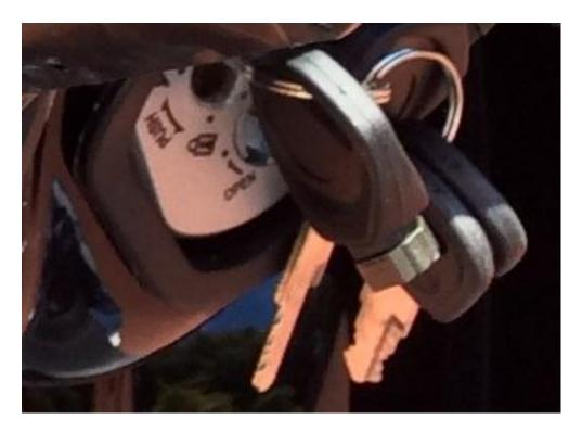
The ignition can be locked to prevent theft and can be opened by the shaped nut on the key.
