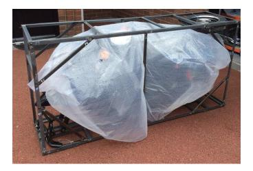
The frame can be dismantled by removing the bolts holding it together with a crosshead screwdriver
