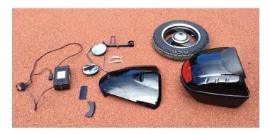
Here's what you should have- charger, mirrors, side stand, stand springs, front trim, front wheel, back box, chassis number cover plate and headlight trim
