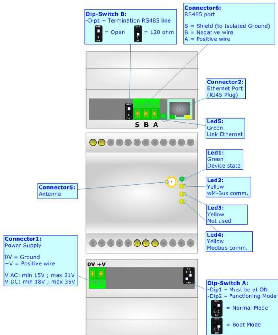
Figure 1a: Connection scheme for HD67082-B2-xxxMHz-0
