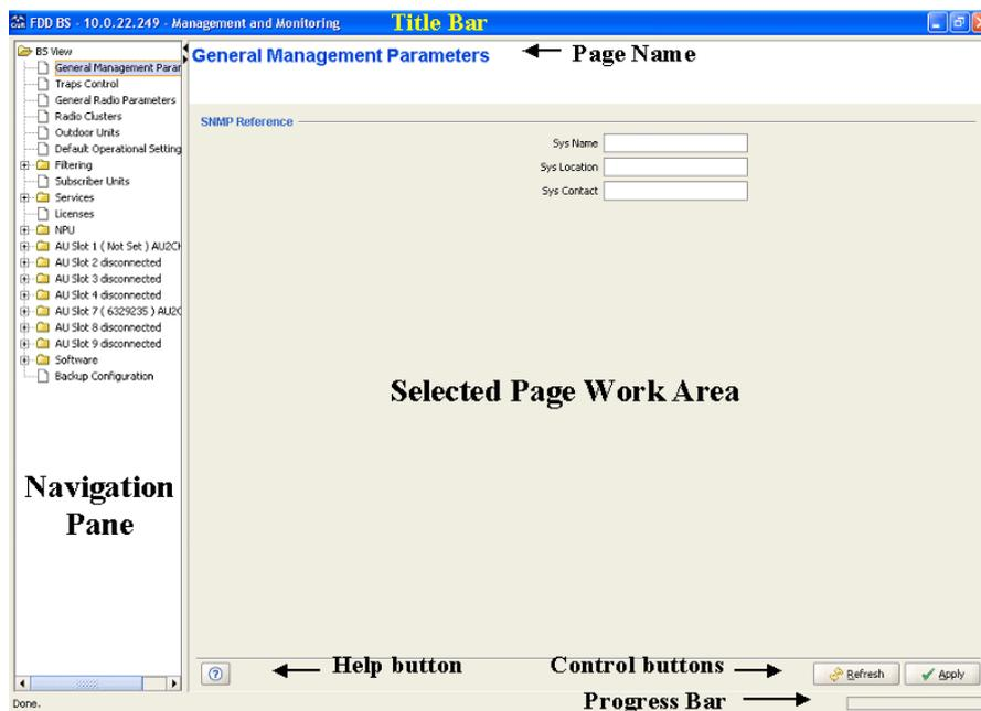
Figure 1-4: The Device Manager Window
