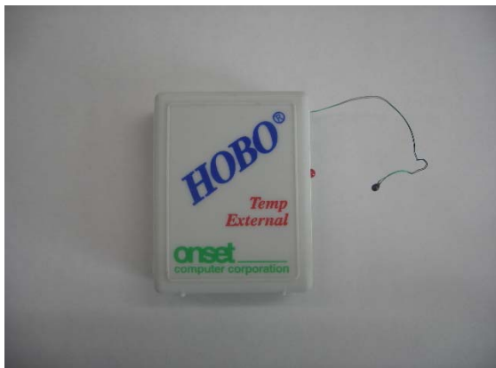
Photo 3.3-1 HOBO by Onset (thermistor thermometer).
