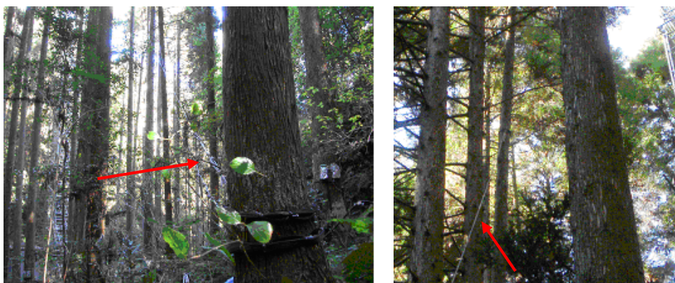
Photo 1.2-5 Trees connected by steel wires at the base (left) and at 10 m (right). The red arrows show the connections. (Kahoku Experimental Watershed)
