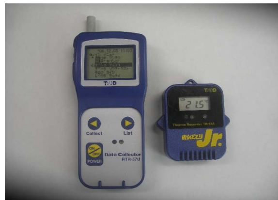
Photo 3.3-2 Ondotori by T&D (thermistor thermometer).
