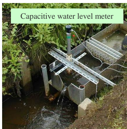
Photo 3.8-2 An example of drainage discharge measurements with the use of a tank style weir (triangular weir). (Mase paddy flux site)
