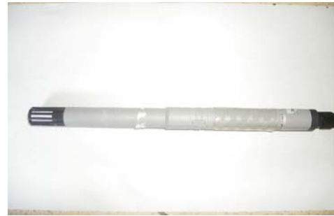
Photo 3.3-3 HMP45D of Vaisala (platinum thermometer, discontinued model, replaced by HMP155).
