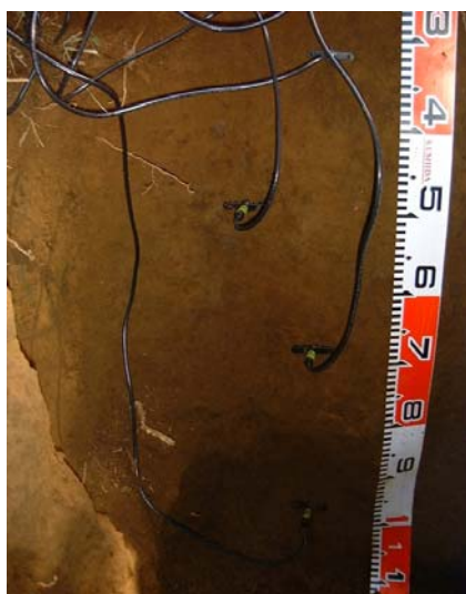
Photo 3.6-3 Soil profile created for the installation of a soil moisture meter EC-5. (Terrestrial Environment Research Center, University of Tsukuba, Photograph: courtesy of Shinichi Iida, FFPRI)
