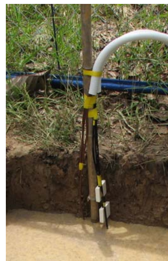
Photo 3.5-4 Underground section where a thermocouple thermometer (left of the stick) and a soil moisture meter (right of the stick) are embedded. (seasonal forest of Kratie, Cambodia)
