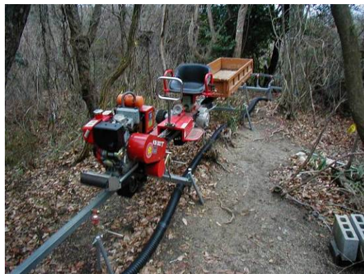
Photo 1.2-4 Monorail used for transporting construction materials. (Yamashiro forest hydrology research site)
