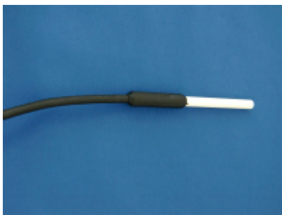
Photo 3.5-1 Thermistor thermometer 107-L, Campbell. (Photograph: courtesy of Climatec, Inc.)
