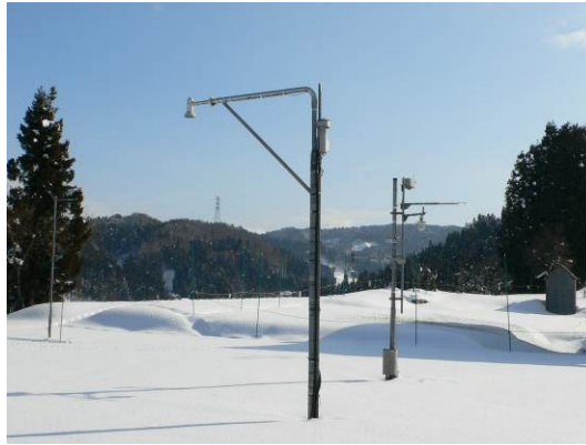
Photo 3.7-2 Snow depth measured by ultrasonic snow gauge. (Tohkamachi Experimental Station)
