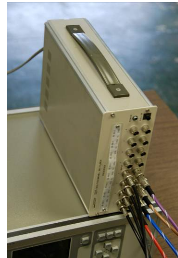
Photo 2.7-1 Low-pass filter for signal cables.
