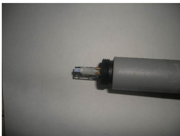
Photo3.4-1 A thin-film polymeric humidity sensor and a platinum resistance thermo sensor in HMP45D (Pt100).
