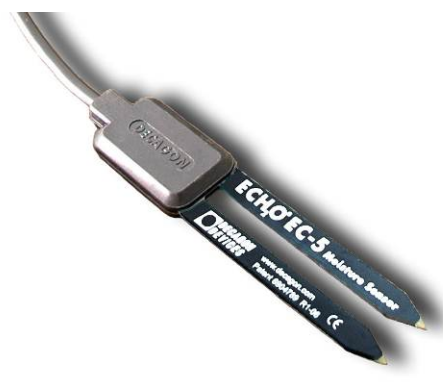
Photo 3.6-1 Permittivity moisture meter EC-5, Decagon. (Photograph: courtesy of Decagon Devices, Inc.)
