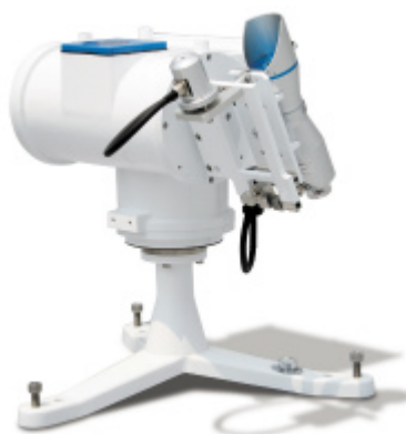
Photo 3.1-2 Pyrheliometer MS-56, EKO equipped with Solar tracker STR-21, EKO.
