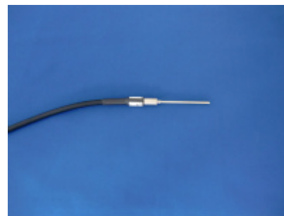
Photo 3.5-2 Platinum resistance thermo sensor C-HPT-5-JM, Climatec. (Photograph: courtesy of Climatec, Inc.)
