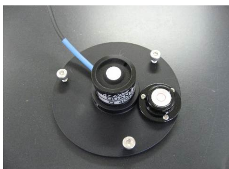
Photo 3.1-7 Quantameters. Left: LI-190, LI-COR. Right: ML020P, EKO.
