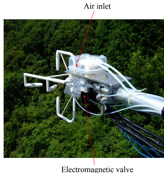
Photo 2.5-1 A SAT and an air inlet used in an REA system. (Yamashiro forest hydrology research site)
