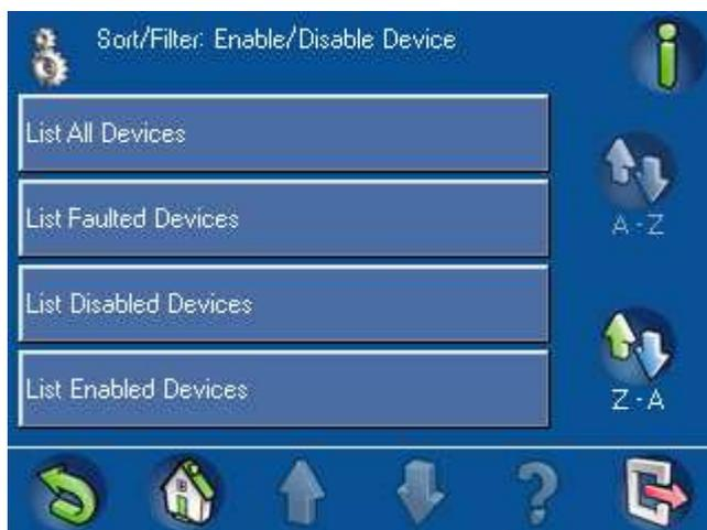
Press one of the device buttons to view additional details of that device. A **View Device Status Detail** screen (Figure 2.58 View Device Status Detail screen, page 40) opens showing the details for the selected device.
