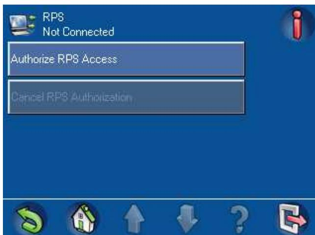
To allow a remote RPS connection to the control panel, press **Authorize RPS Access**. To cancel the authorization for a remote RPS connection to the control panel, press **Cancel RPS Authorization**.
