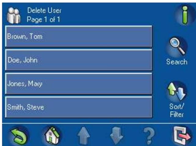
From the **Delete User** screen, press one of the menu buttons containing a user's name. A message appears asking for confirmation (Figure 2.34 Confirm Delete User screen, page 29). To proceed, press the **Confirm Delete** button. If you do not want to delete that user, press the **Back** button.
