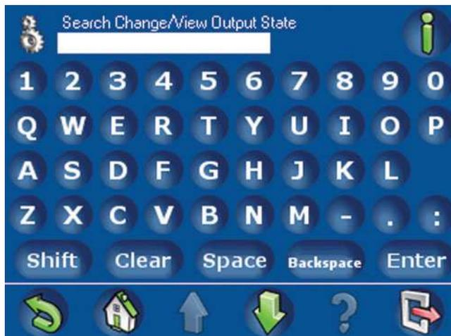
To sort or filter the list of outputs, press the **Sort / Filter** button on the **Change / View Output State** screen. The Sort / Filter Change / View Output State screen (*Figure 2.95 Sort / Filter: Change / View Output State screen, page 58*) opens.
