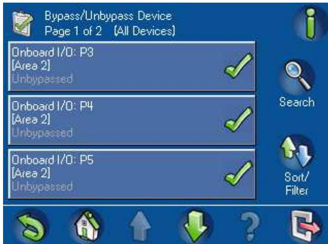
To find a specific device, the user can search or sort the list. Press the **Search** button to show the Search Bypass / Unbypass Device screen (Figure 2.60 Search Bypass / Unbypass Device screen, page 42). Use the numeric, alphabetic, and command keys to enter a device's name. The name appears in the **Search Bypass / Unbypass Device** field. Press the Enter button to start the search.
