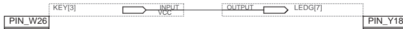
Figure 1.4 A simple circuit that connects pin W26 of the FPGA to pin Y18 of the same chip. Since this circuit simply passes a signal through the device, none of the logic elements (LEs) will be used!
