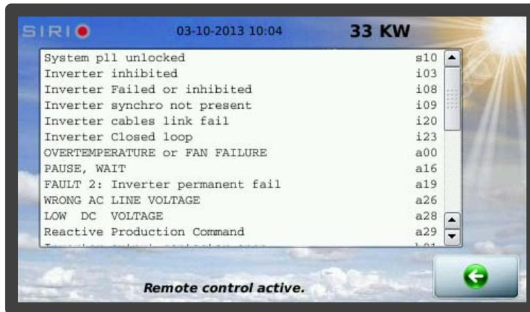
You can use your finger to scroll through the list of any alarms. Remember that in the event of an alarm, a sound will be emitted at 5-second intervals until the alarm disappears or the user touches the screen. If the user touches the screen, the sound will change intensity and timbre. If after 20 minutes the user has not deleted the alarm, the sound will go back to the original one.
