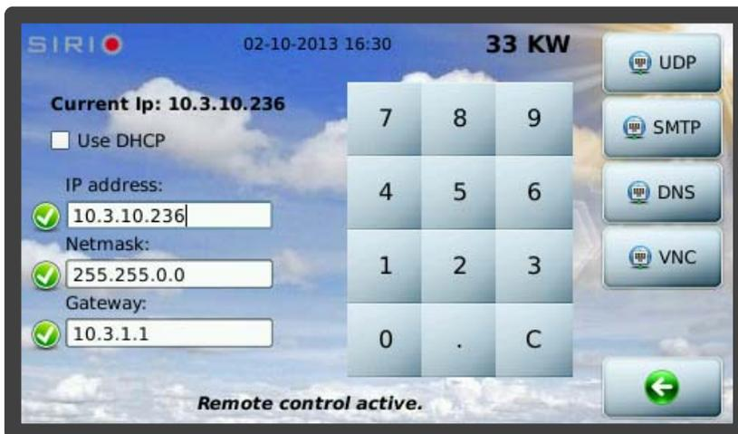
The IP address may be assigned statically, as in the previous figure, or can be obtained through a DHCP server. Touch the selection box to choose this setting:
