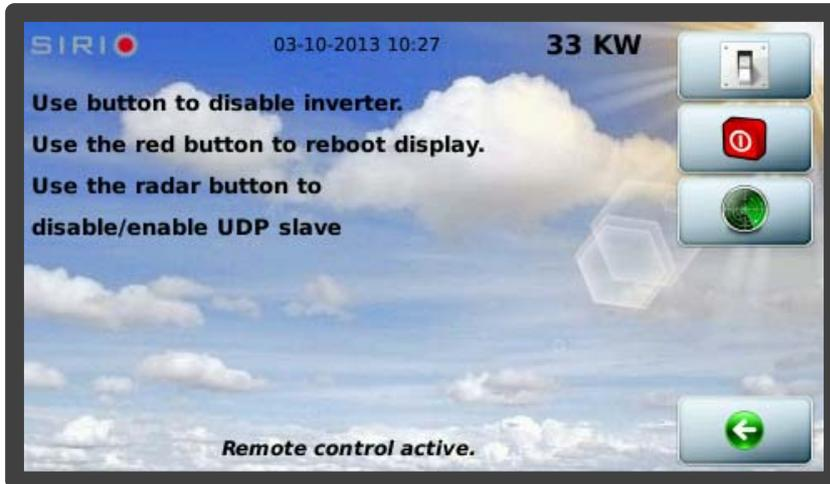
The first button allows you to disable the inverter and re-enable it. The second button allows you to restart the graphical interface for any display software updates. This action does not affect inverter operation in any way.
