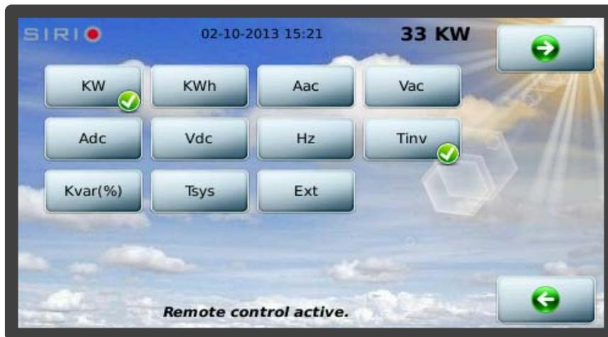
To select a measurement, press the corresponding button. A white tick will appear on a green background to highlight the choice.
