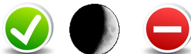
The first symbol indicates that inverter operation is regular, the second that solar radiation is low and the third indicates an alarm.
