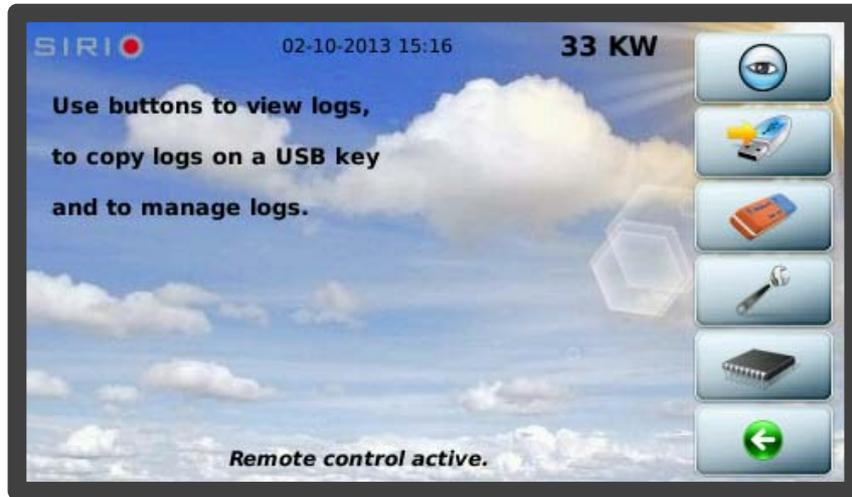
To view the logs, press the button with the
