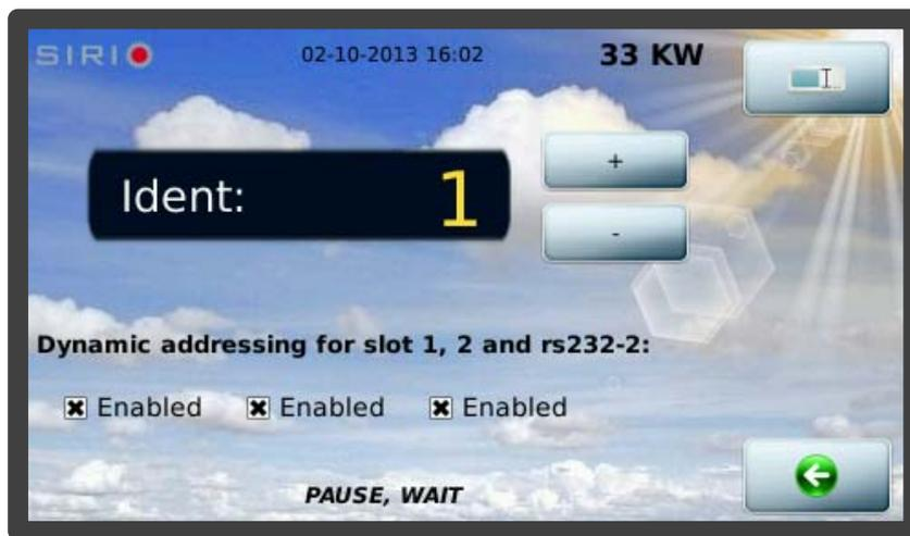
In the same window, we see that for each serial port, it is possible to specify whether the addressing is dynamic or static<sup>1</sup>; this is a technical issue that regards the compatibility of communication protocols. In particular, this configuration data concerns the PVSER protocol (Proprietary Protocol).
