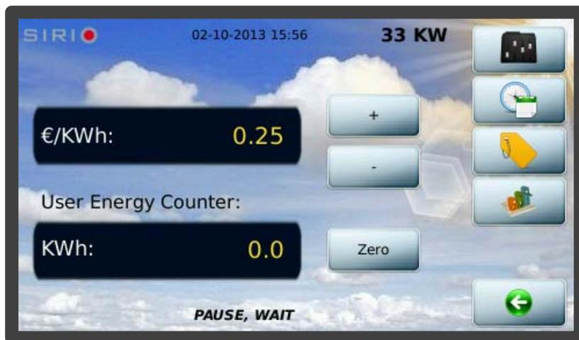
On this screen, you can manually set the €/kWh ratio and reset the partial hour meter for the energy produced.
