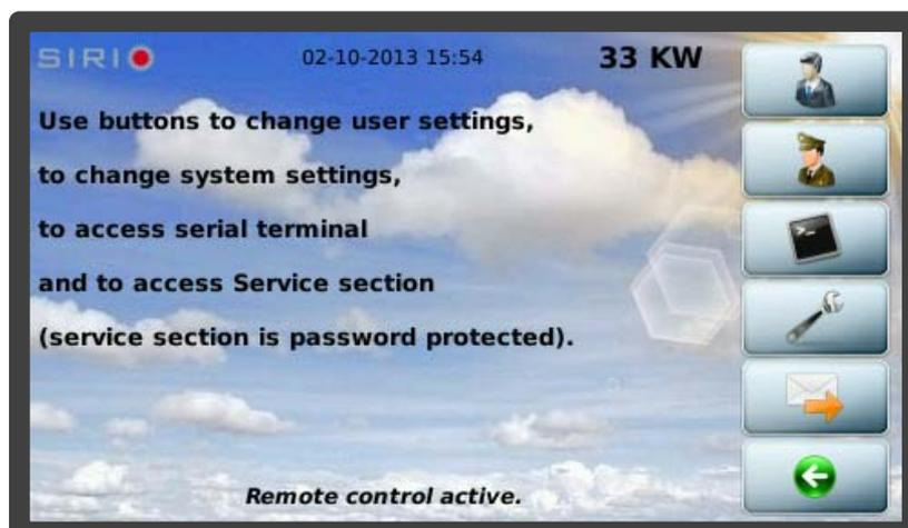
Once again, on the right, there are additional buttons which, from the top downwards, can be used to set user parameters, system parameters (do not require a password but an in-depth knowledge of network issues) and to access terminal mode for low-level interaction with the inverter.
