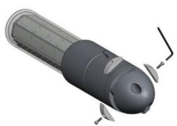
Use a 5mm Unbraco key to release the screws, then remove and change the anodes. Refasten the screws.
