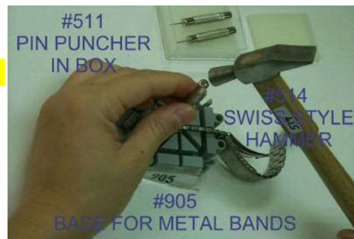
T-905 METAL BANDS OPENING BLOCK FOR HOLDING METAL BANDS ON ADDING AND DELETING LINKS
