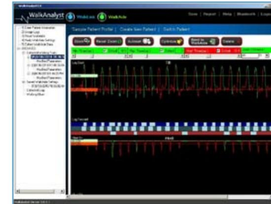
Figure 72: The On Threshold is set too high, producing a delayed pattern of stimulation
