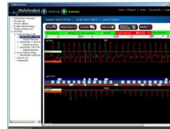
Figure 73: The Off Threshold is set too low, below the Tilt graph data
