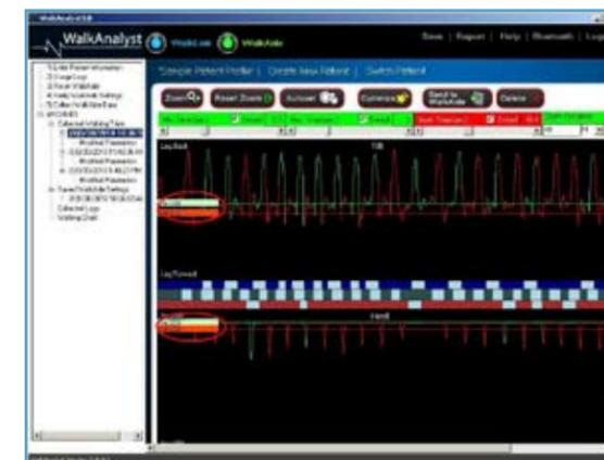
Figure 70: Adjusting the On and Off Thresholds
