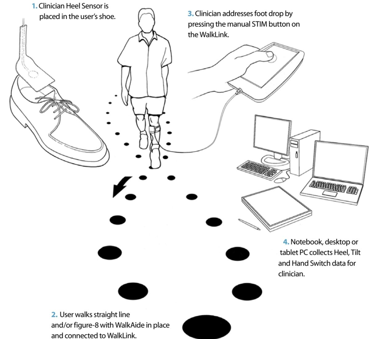
**Figure 2: Initial WalkAide set-up procedure using the WalkLink, Heel Sensor and WalkAnalyst software.**
