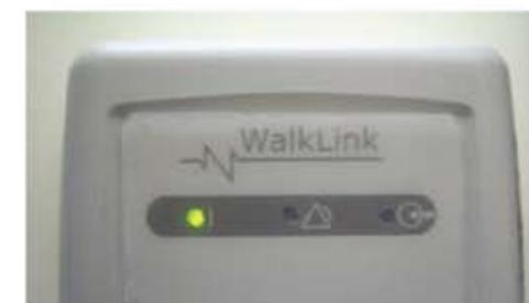
Figure 18: Flashing green light indicates WalkLink is on
