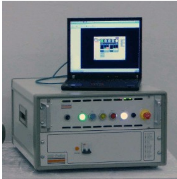
NSD Central Control Unit and 1.8 kW DC HV PSU enclosure. A typical industrial PC and its I/O modules plus power switching relays and 24 volt DC power supply can be accommodated in a 3U 19" sub-rack or similar enclosure.
