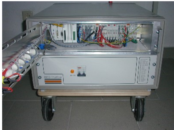
NSD Central Control Unit and 1.8 kW DC HV PSU enclosure. A typical industrial PC and its I/O modules plus power switching relays and 24 volt DC power supply can be accommodated in a 3U 19" sub-rack or similar enclosure.
