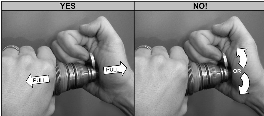
6. Use the swirl ring removal tool (P/N BK260105) to remove the swirl ring from the nozzle.
