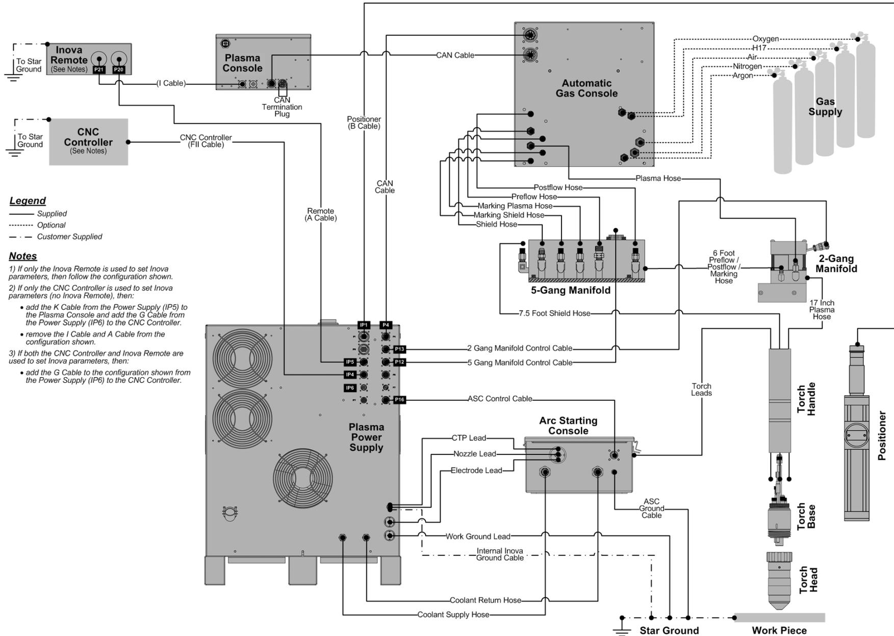
Figure 1c: Spirit II System (AGC, Internal Inova, ASC with CleanStrike™ Technology)
