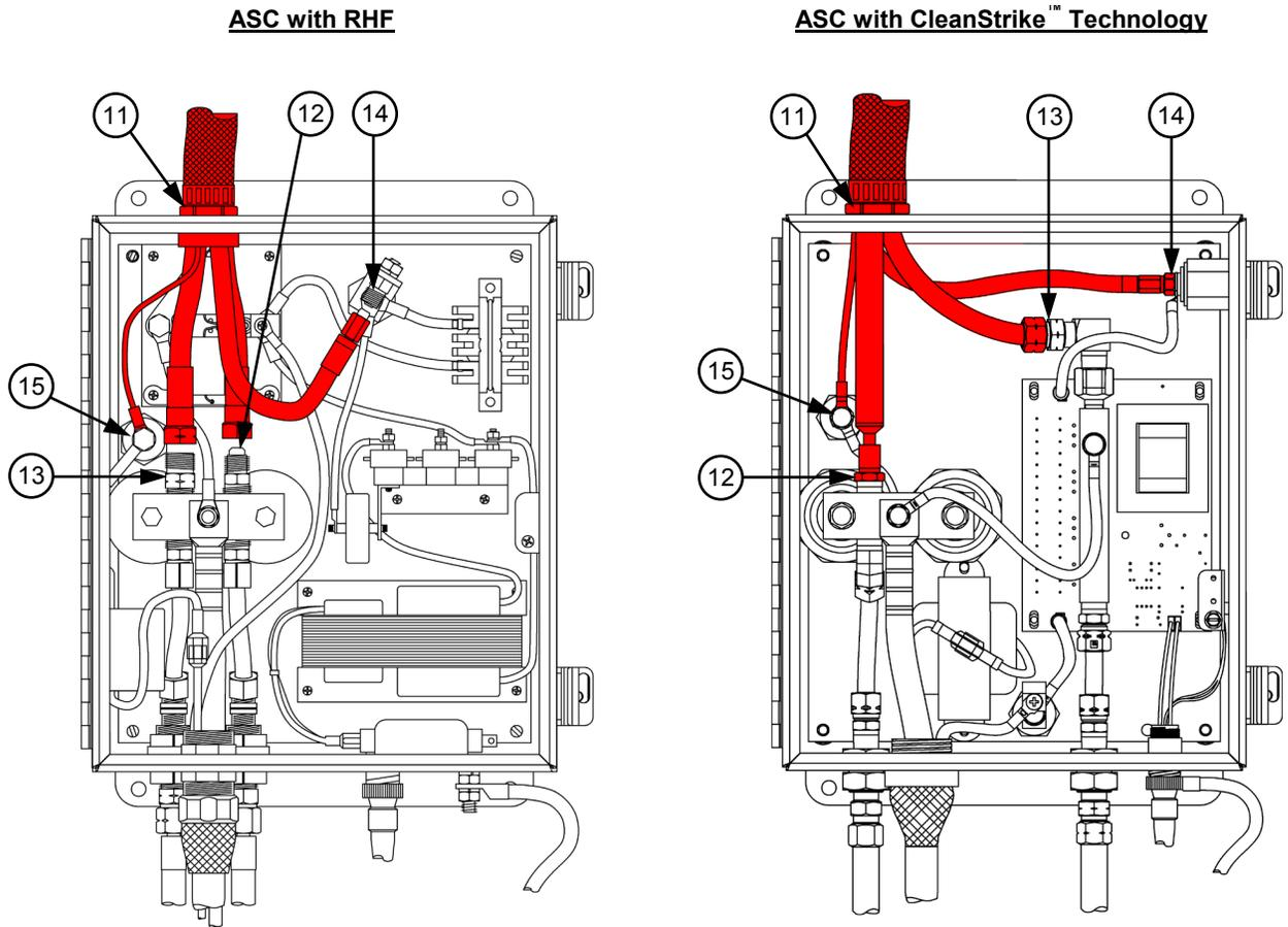
**Figure 6: Torch Leads to Arc Starting Console Connections**
