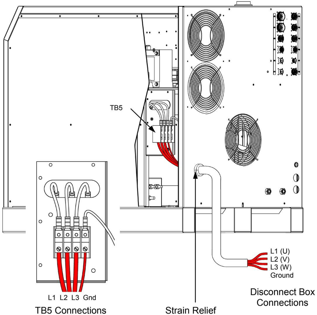
**Figure 3: Power Supply Primary Connections**
