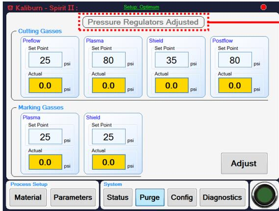
A message at the top of the screen indicates the status of the regulators in the automatic gas console:
