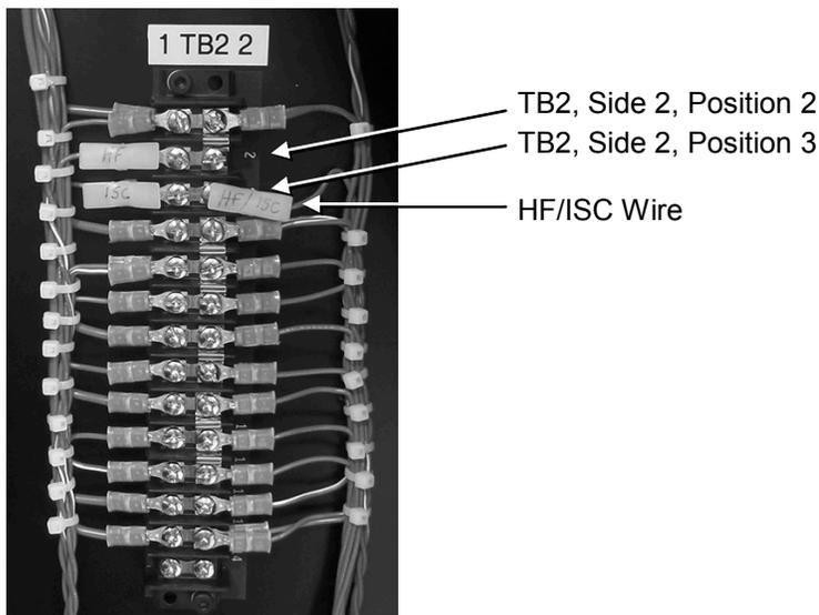
4. Remove the Electrode, Work and Nozzle leads from the output terminal block, which is located on the left side of the unit.
