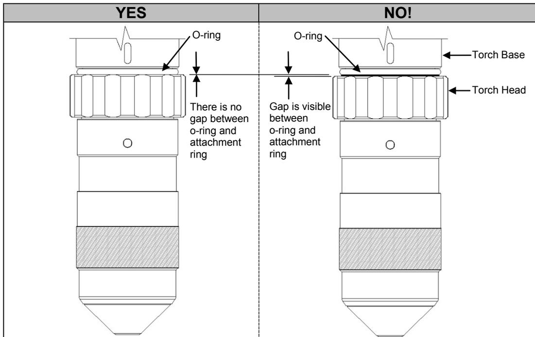
To remove the torch head, turn the attachment ring to the LEFT.
