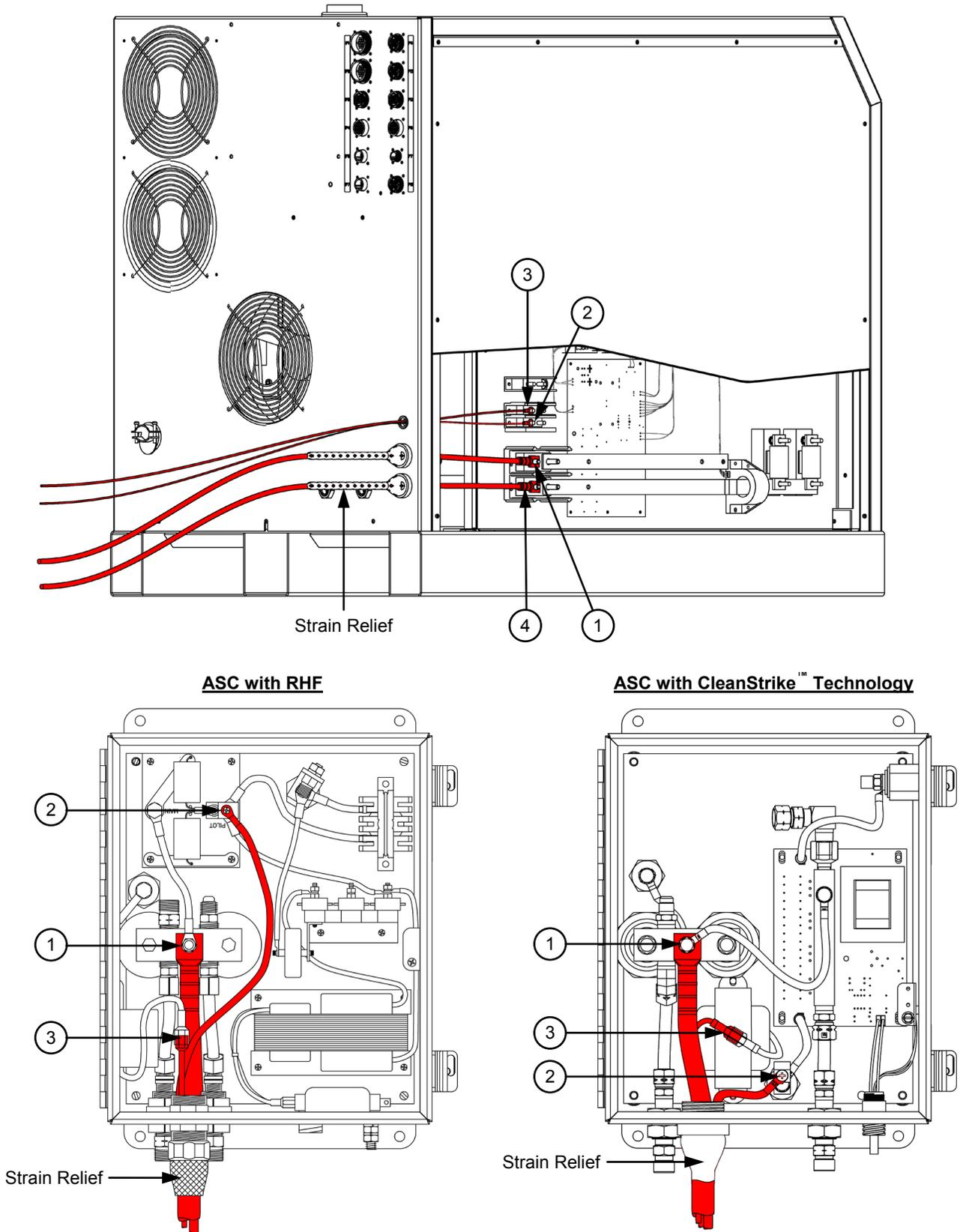
**Figure 4: Power Supply Output Connections**
