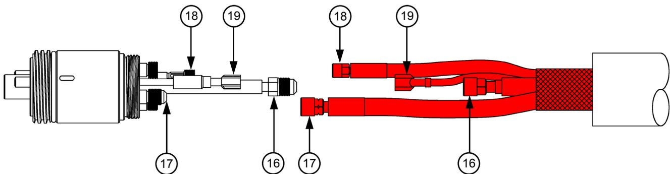
**Figure 7: Torch Leads to Torch Base Connections**
