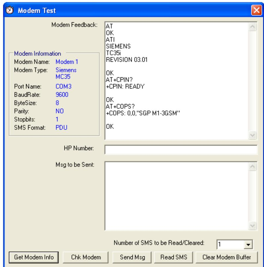
**Figure 20: Modem Test Interface**
