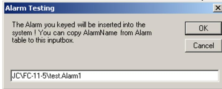
Notes: If you insert the same alarm twice into the system, they won't be handled as 2 alarms, only the last occurred alarm will be inserted into WaitQ (use the last alarm occurring time to update the AT field). This design also applies to real alarms from OPC.
