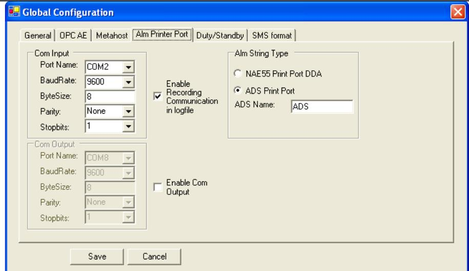
**Figure 6: Global Parameter (Alm Printer Port) Configuration**
