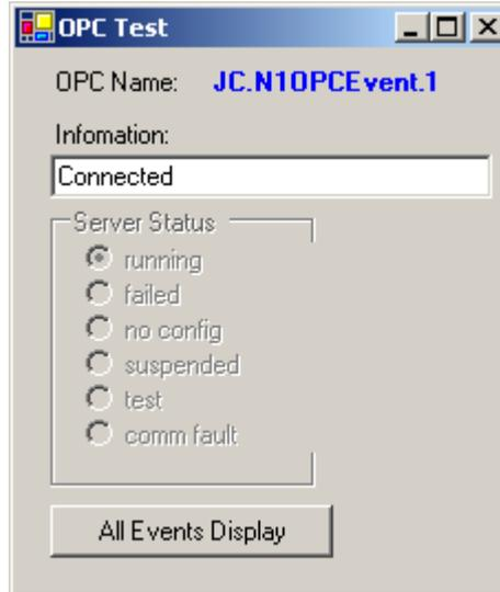
**Figure 22: OPC Test Interface**
