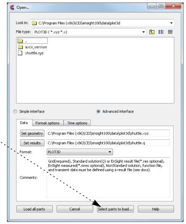
When the File Selection dialog is closed, EnSight reads the indicated file but does not load any of the geometry.
