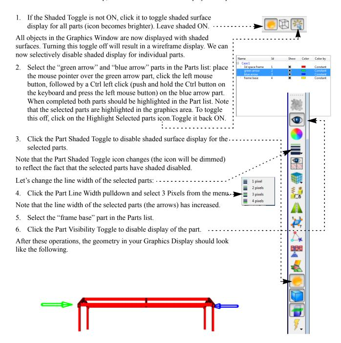
Parts are assigned a default color when loaded into EnSight. These colors are *constant*, meaning that every portion of the part is colored the same. Parts can also be colored by a variable value. Since the value associated with a variable typically varies from node to node, the displayed color will vary across the surface of the part.
