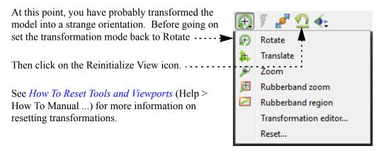
You can also perform precise transformations (such as rotating 22.5 degrees about the X axis) using the Transformation Editor
