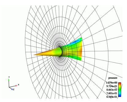
The new "Clip\_plane" part listed in the Parts list has attributes just like the original model parts. For example, we can color the part based on the value of a variable and change other attributes as well (like we just did with its visibility).
