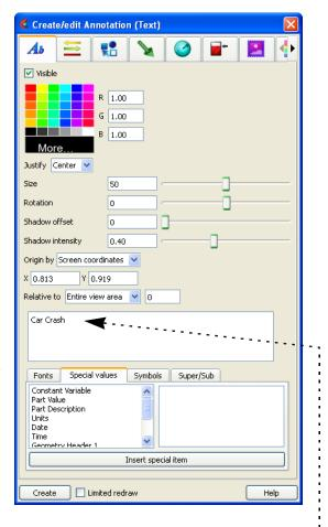
EnSight supports several "special strings" that let you automatically display constant variable values as well as various internal values. For example, you can have a text string that displays the current solution time. When the time step is changed, the text automatically updates.
