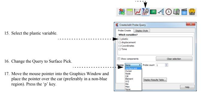
The value of the plastic strain variable is calculated for the point under the mouse and displayed. A marker (the sphere) is also displayed.
