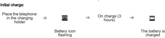
Maximum battery performance is only reached after around 10 charge/discharge cycles. These batteries contain polluting substances: do not dispose of them in a dustbin - take them to a specialized collection point.
