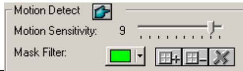
**Motion Detect**— If you have this selected, the QuikCam software will only record if it senses any movement occurring in the area the camera is pointing toward. This setting also features sensitivity controls, 10 being the highest. As level 10 is too high for normal use, this is preset to 9.
