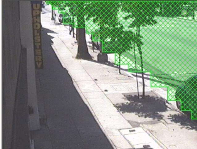
In the example above, we have masked off the street, but any motion on the sidewalk, will trigger the motion detection to start recording.
