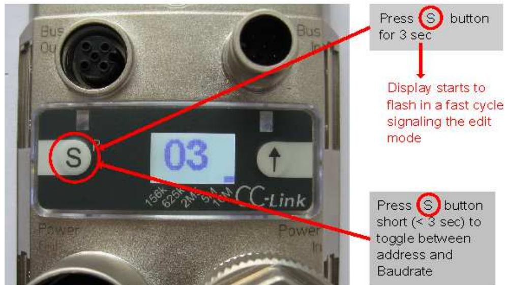
The BNI CCL-502-100-Z001 serves as a decentralised input/output and IO-L master module for connecting to a CC-Link network. With the implemented display, the address, the communication speed and the CCL mode preset is set directly on the BNI CCL-502-100-Z001 devices.
