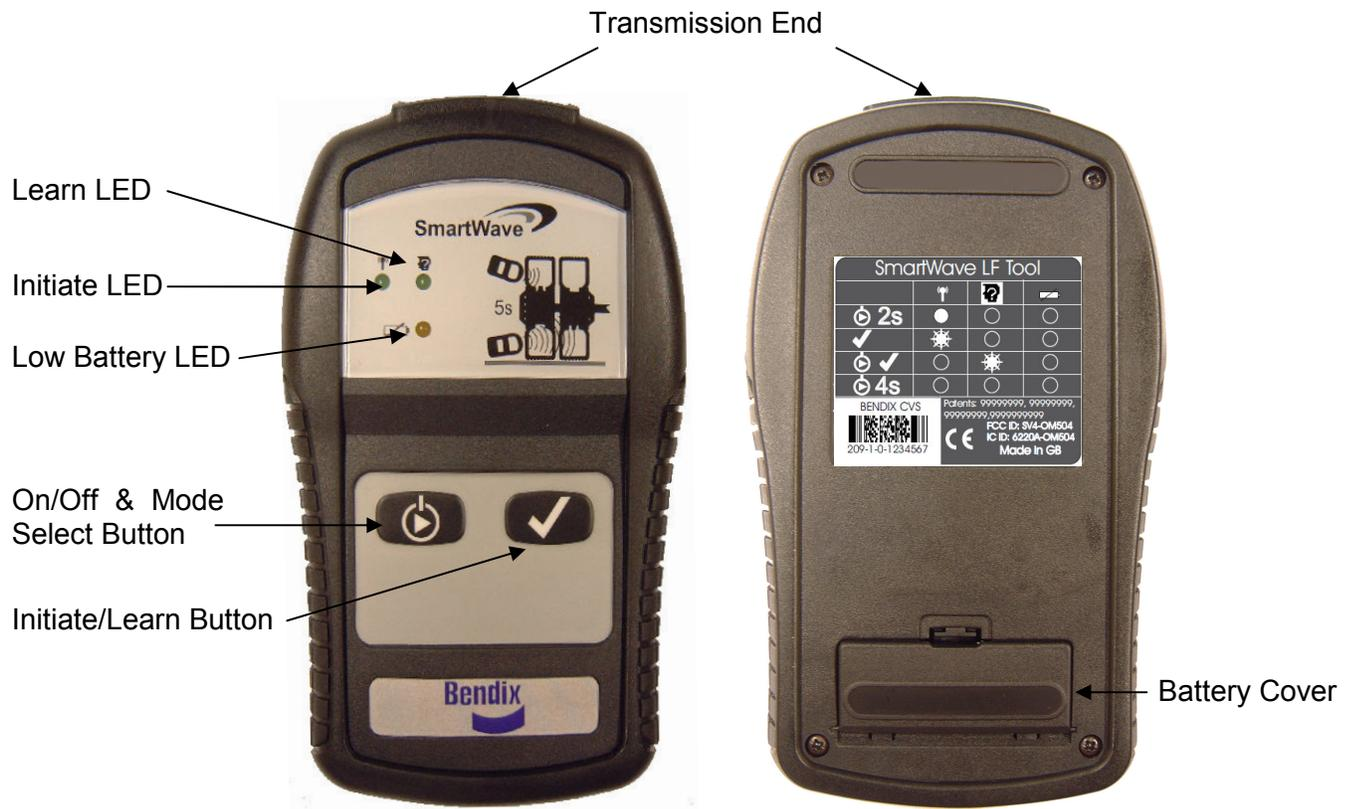
**Transmission End:** This part of the tool must be pointed towards the tire to initiate or learn a sensor.
