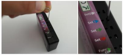
**Pressing SetC on an RC4 Series 3 DMX4dim.** The DimC indicator is behind the round hole. The button is behind the slotted hole. With a DMX channel set higher than 20%, press the SetC button and the DimC indicator will come on. Dimmer C is now assigned to that channel.
