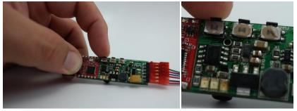
**Pressing SetB on an RC4 Series 3 DMX2micro.** The DimB indicator is on the opposite side of the device, near the DimB pins on the multipin power connector.
