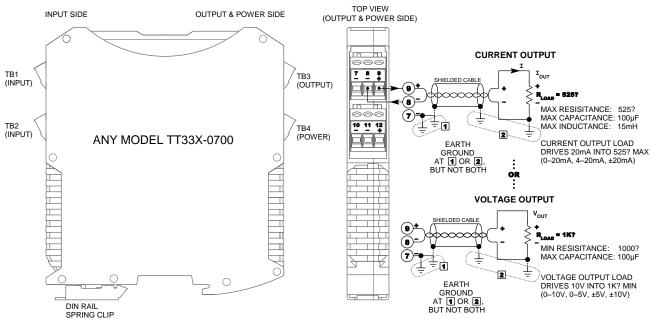
Observe proper polarity. Note that twisted-pair wiring is often used to connect the longest distance between the field transmitter output and the remote load as shown above. Additionally, shielded twisted pair wiring is recommended for best results. An output connection to earth ground will help protect the circuit from damage in noisy environments.
