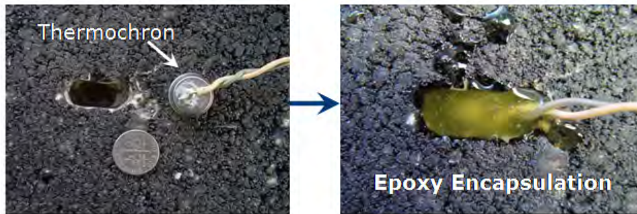
Figure D.1. Thermochron embedded in asphalt pavement
