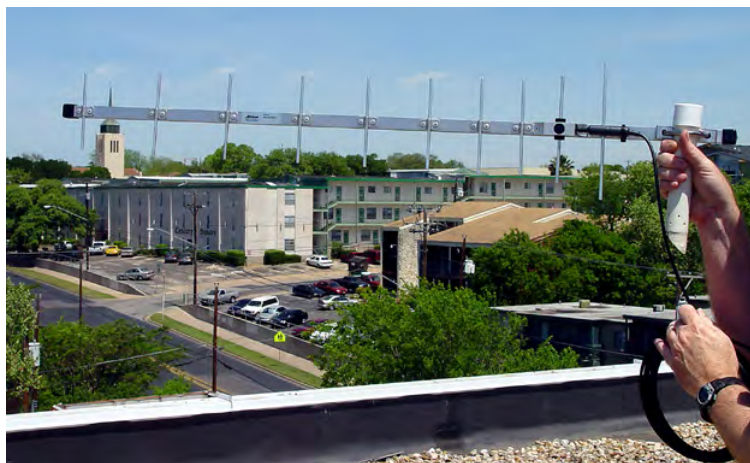
Figure 4.11: Yagi directional antenna with 22-mile range (line-of-sight)
