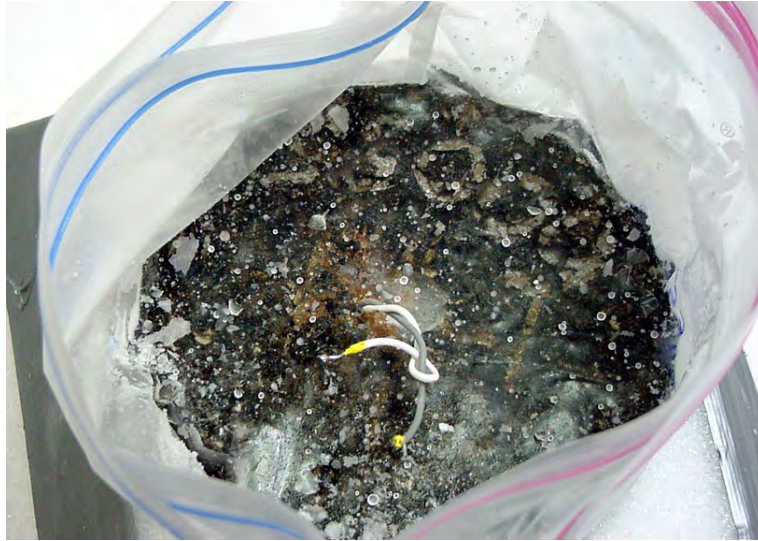
Figure 4.6: Black ice formation in one of the NGOGFC laboratory specimens
