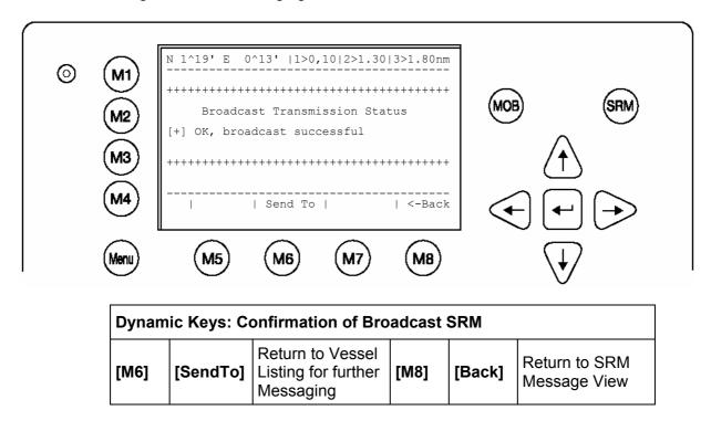
After pressing [SendTo] from the previous screen, the user is taken back to the Vessel Listing for the option of writing further addressed messages.
