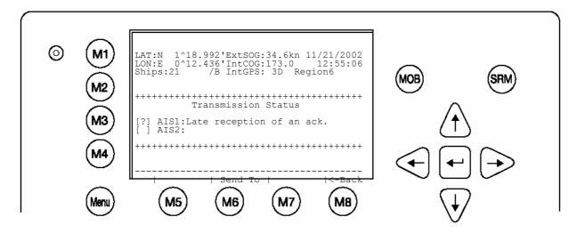
It is possible, that the recipient's Transponder could not receive the message at all, and in this case the following screen is displayed. It is then recommended to resend the message.
