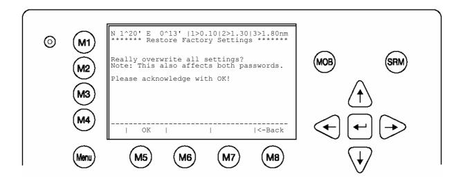
After pressing [OK], the Data Saved Screen confirms the Restore Factory Settings command.
