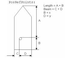
The RM808 AIS automatically calculates the missing distances (a) or (b) and (c) or (d) - based on the vessel's length and beam.
