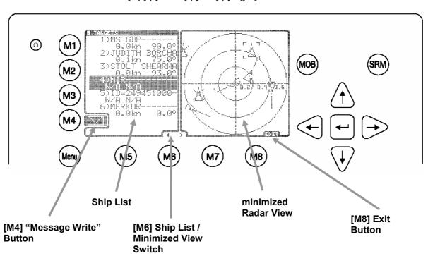
Radar View → [Up] | [Down] | [Left] | [Right] → Minimized Radar View
