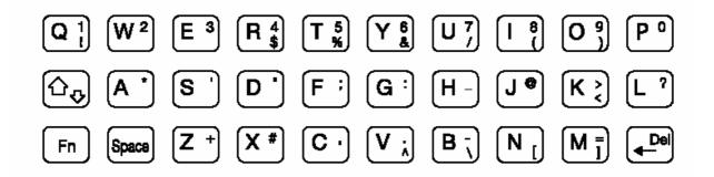
Tip: The RM808 AIS automatically changes the keys "Q" through to "P" to numerical input when the current application requires numbers, rather than letters to be input. This feature is enabled when [NUM] appears on the bottom left hand side of the screen.
