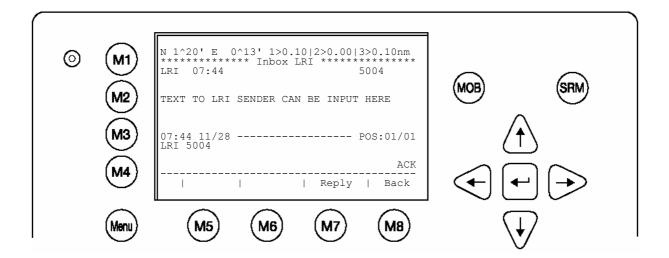
An LRI has arrived; the RM808 AIS Settings are configured to **Manual Mode**: The LRI therefore needs to be manually handled (accepted or rejected)
