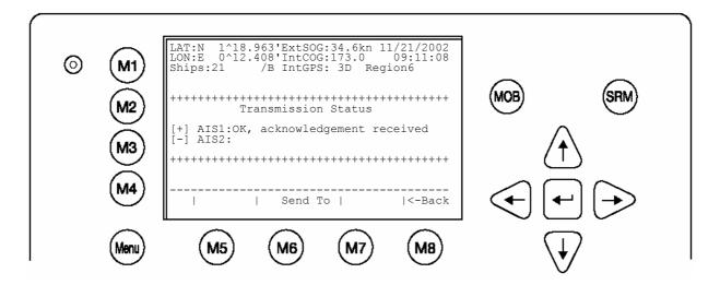
In some cases, the recipient's Transponder may not be able to receive the message immediately – due to Transponder in-operation. In this case, the confirmation of the send message arrives later, upon Transponder re-operation.
