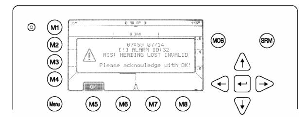
Pressing [M5] leads to alarm acknowledgement and the closure of the window as well as the alarm icon disappearing. An alarm could occur at every time so the alarm icon can be seen in **every** view (in the big views as well as minimized views and ship details list).
