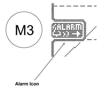
Pressing the [M3] button shows the details of the selected alert.
