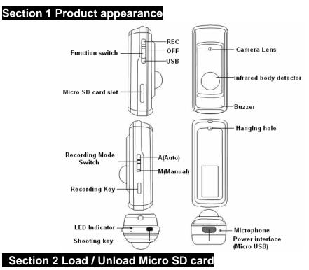
Allocating the card slot at the left side of device, make sure the card pin contacting on down side and slide the card into the slot until it clicks. Push the Micro SD card until you hear a click, then release.
