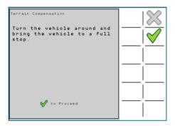
5. To proceed with the Terrain Compensation setup, select . The operator is instructed not to move the vehicle as tuning of the sensors is in progress.
