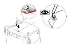
Remove the protective strip of the double-sided tape on the bottom of the GPS antenna.
