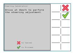
When you are driving at 4 km/h and are ready to proceed with the steer kit calibration, select the button. The next steering calibration screen appears.
