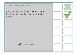
7. To proceed with terrain compensation, select . The operator is instructed not to move the vehicle as tuning of the sensors is in progress.
