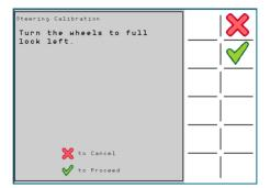
To proceed with the steer kit calibration, select the  $\checkmark$  button. The Progress of Adjustment screen appears showing the progress of this stage of the steering calibration.
