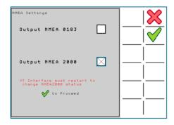
5. To complete the NMEA 2000 Settings setup by allowing the restart to occur, select ✓.
