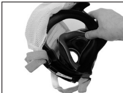
FIGURE 3 Checking Voicemitter Ducts
