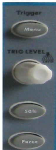
**Fig.4-14** Trigger Control Zone
