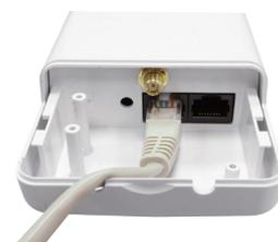
**STEP 3:** Slide the cover back and insert the protective plug to seal the bottom of the WNAP-6305.
