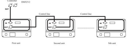
Caution: Please remember the signal output of last machine must connect the attached circle plug .The circle plug connect a 120 resistor between 2 feet and 3 feet canon plug. The signal reflects phenomena can be avoided by using circle plug during DMX 512 signal transfer.
