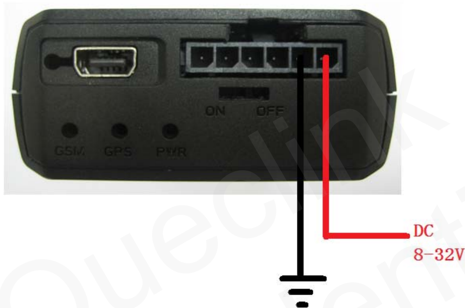
Figure 8. Typical Power Connection
