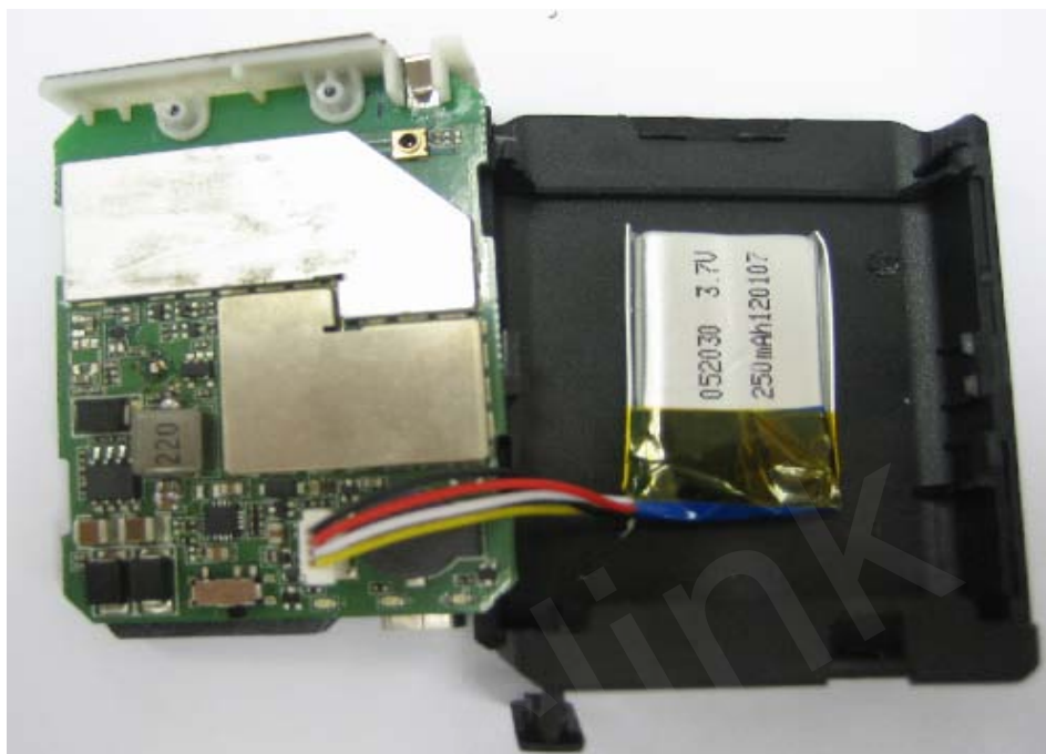
Figure 6. Backup Battery Installation
