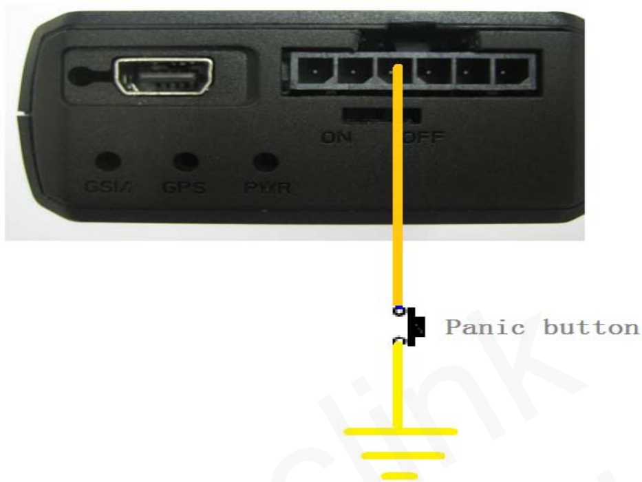
Figure 10. Typical Digital Input Connection
