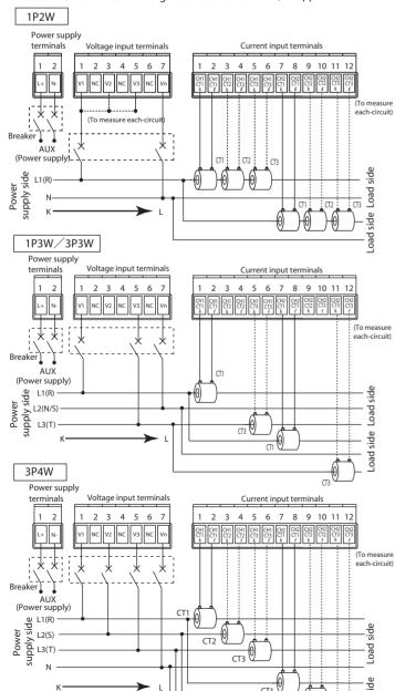
⚠ Vn terminal should be connected to N-phase which is grounded.
