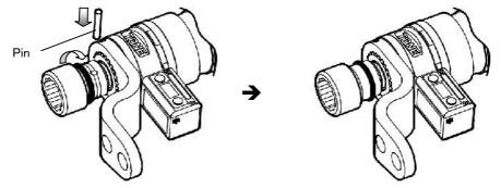
(5) Check that the O ring is properly attached, and also make sure that the socket does not come loose from the main unit.
