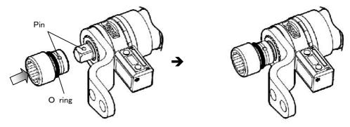
4 Attach the pin to the socket pin hole so that the pin does not come out, attach the O ring in the groove.
