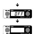
NOTE "Automatic display shut OFF mode" starts again if there is a 10-minute pause without any operation after releasing "automatic display shut OFF mode".
