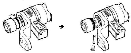
2 Remove the socket from the output angle adjustor.
