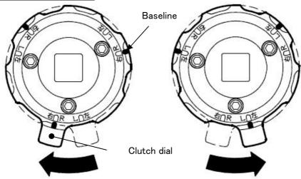
When rotate clockwise, adjust the baseline to Right (R).
