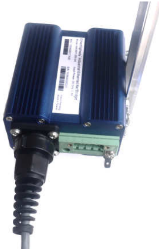
Figure 2.4.2 – Ethernet Cable on AIA1803-200-04 RJ45 port
