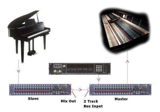
Sometime the console being used for a mix simply does not have enough inputs. This may be because it is a small digital mixer being used to meet a fixed budget or because the console has a limited number of inputs.
