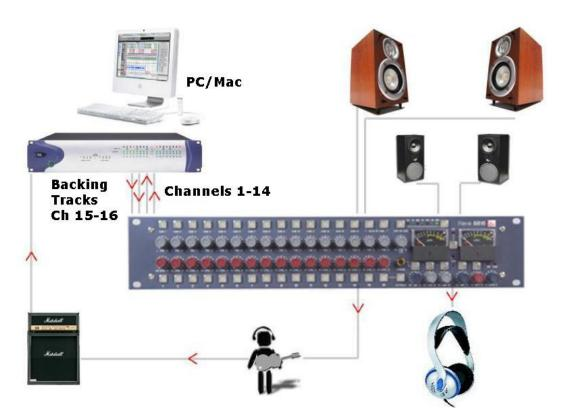
Connect the outputs of the workstation to the inputs of the 8816. If you have a backing track pre-mix on your workstation assign this to outputs connected to inputs 15/16 on the 8816.
