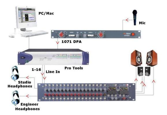
The 8816 can be used to monitor from the workstation while recording directly from a mic pre such as the 1073DPD or as a pre-mixer for recording a number of signals simultaneously to the workstation. With the optional fader pack, direct outs can be used from the 8816 to the DAW enabling it to be used like a conventional desk with both recording and monitoring signals passing through the unit.
