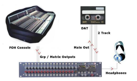
While the output for the main Front Of House console may be of a high standard, the mix created for the venue does not have the correct balance for the recording. The 8816 can solve this problem.
