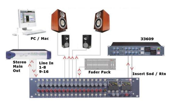
The engineer and producer can monitor on two sets of speakers, main and near field, and switch between them using the **Alt Speaker** switch allowing comparisons of the mix on small and large speakers. Headphones can also be connected if required.
