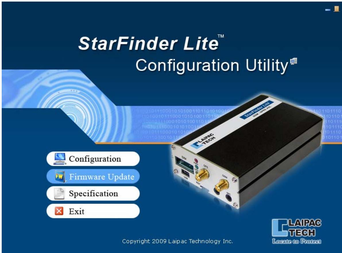
Sometimes we will release new firmware (the program inside the device) which will add new features and enhance others. These updates can be easily performed using the StarFinder Lite Utility once you have downloaded the new firmware file from the website.
